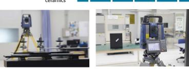
Auto-tracking test under high speed vibration conditions Auto-tracking durability test against rotating object.
