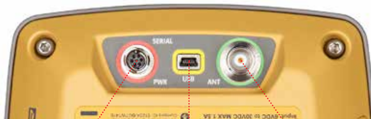
Waterproof Communication and Charging Port
